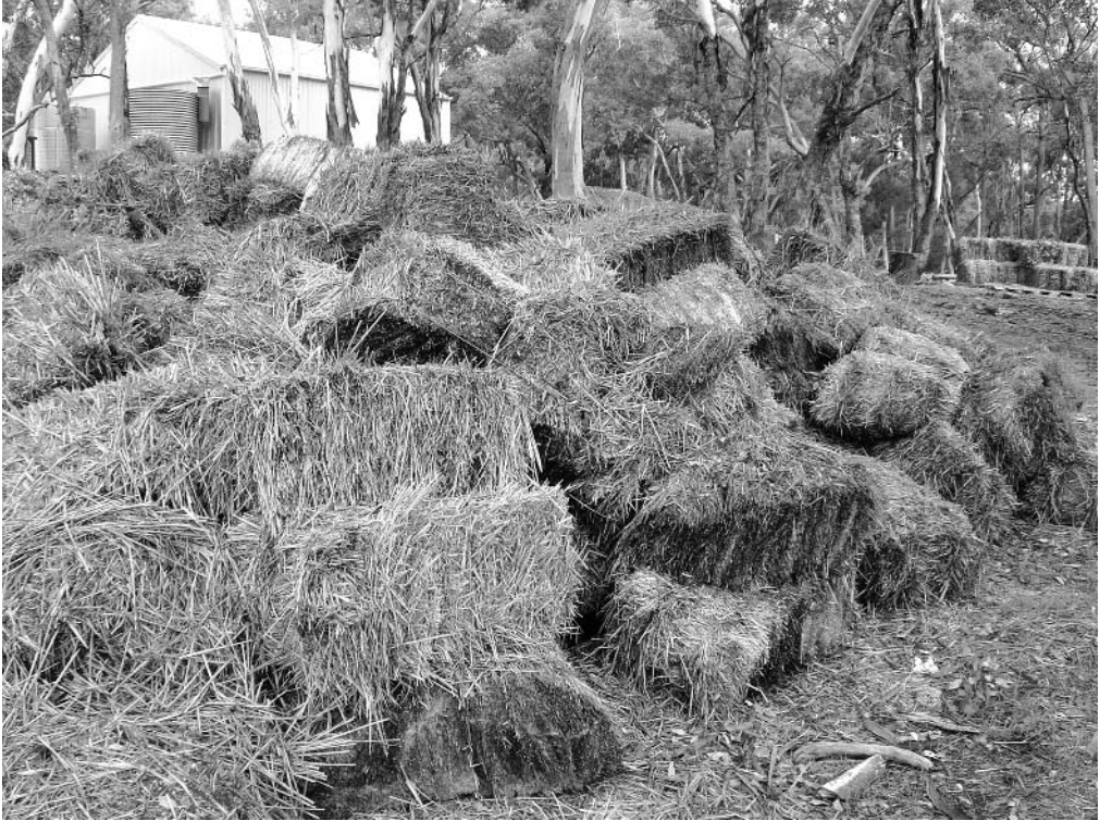
Fig. 31 When bales are not stored correctly they can quickly become useless for building.
