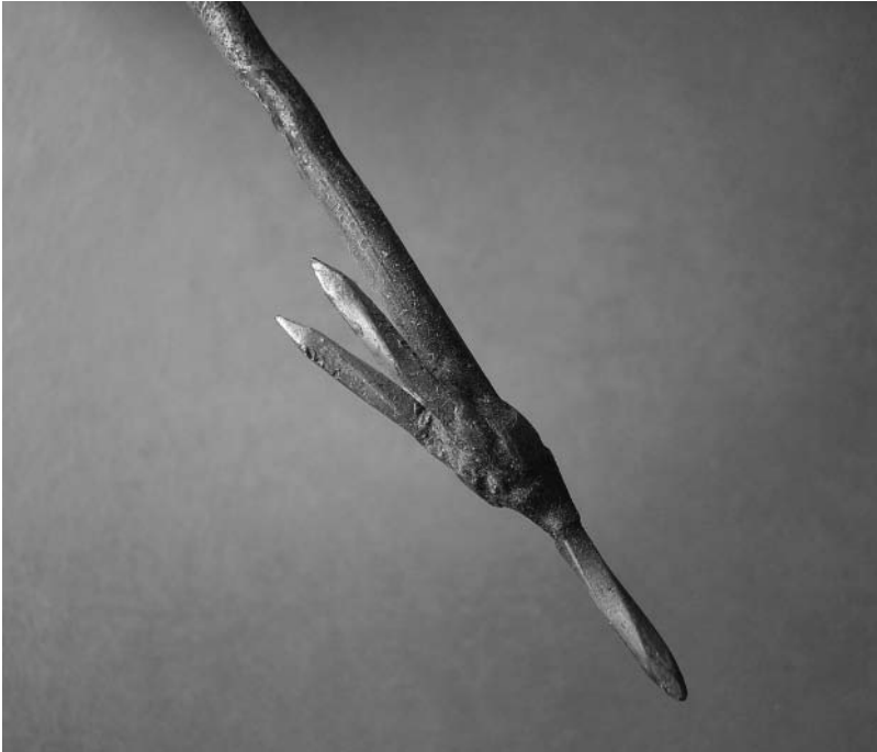
Fig. 10 A 'push-pull extractor' tool, used for extracting straw from a wall to produce holes, such as for pipes. It may be made by welding masonry nails to a steel rod, with a suitable handle on the other end.
