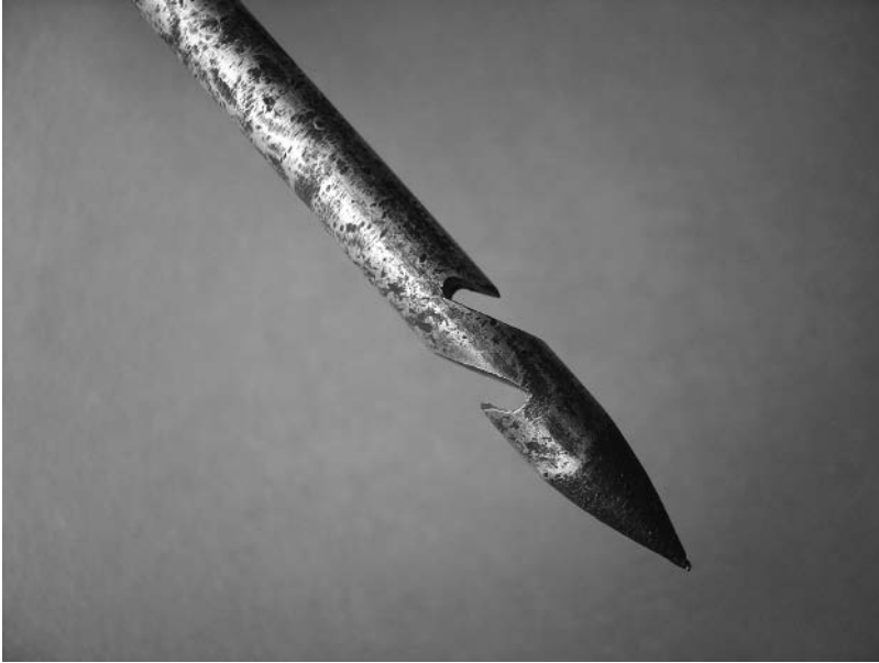
Fig. 9 Needle used for threading twine through a bale when splitting bales. Twine may be inserted by both a push and pull action.
