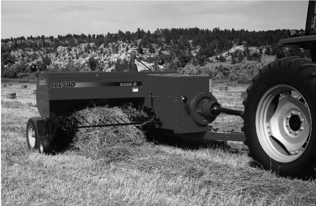
Fig. 3 Baling machine in operation. The rotary rake picks up the straw, and steel fingers move the straw to the right. The ram that compresses the bale, the tying mechanism and the cutters are in the right hand section.
