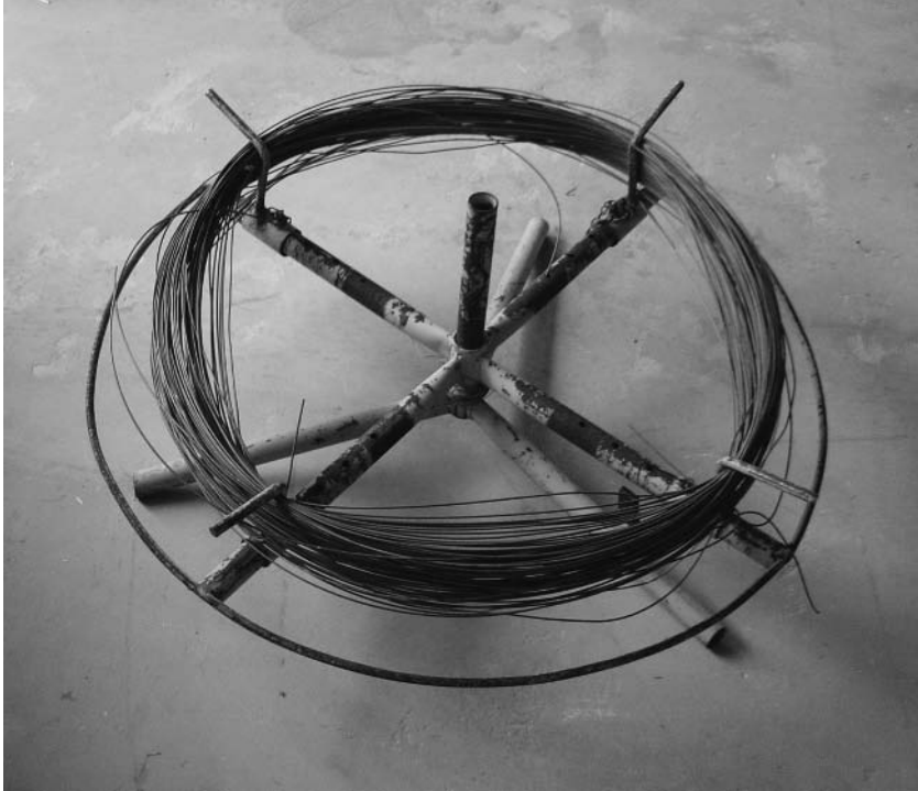
Fig. 12 A wire spinner is essential for working with rolls of high tensile wire to prevent horrendous tangles.
